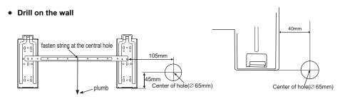
NOTICE: • Confirm the position of holes, and drill holes on the wall.
