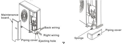
The cable wire can be led from the back hole of the pipinghole or ejectinghole.
